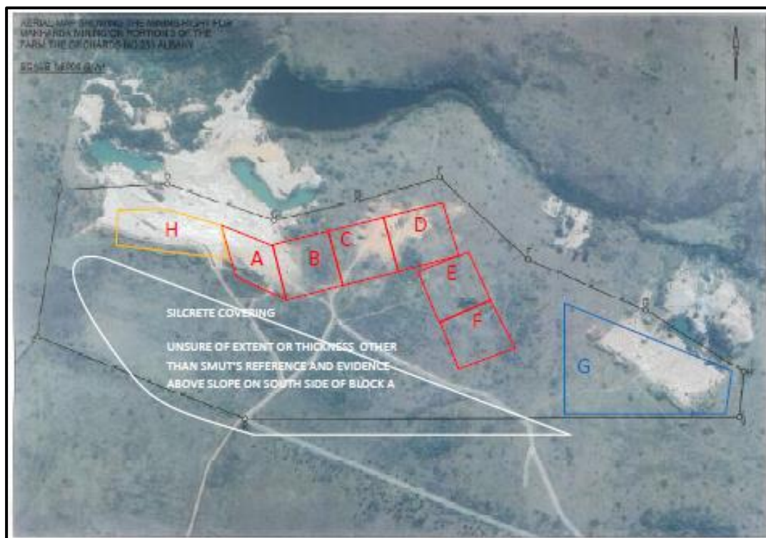
Figure 10: Plan showing the aggregate (silcrete) and clay sources within the earmarked area. Note white, and yellow kaolin in blocks A & H, and Naartjie Red Clay in blocks C & D.
